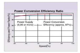
Using VFDs, the reduction in speed leads to the increment in power factor and thereby efficiency gets enhanced upto 96 to 98 percent.
