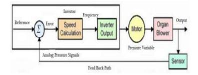
As the supply is given at required frequency, the speed can be adjusted accordingly and wear & tear of motor or electrical equipment can be reduced, leads to the increase in life-span of electric-motors. With the reduction in supply-power-frequency, the power-factor increased significantly which results in efficient energy usage by amplifying its efficiency.
